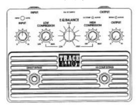
Two LED's indicate the ACTIVE status of the unit, these are EFFECT ACTIVE above the OUTPUT control to indicate when the effect is switched into circuit, and HI COMP ACTIVE to indicate when the HIGH COMPRESSION is switched into circuit. This second LED will indicate the status of the HIGH COMPRESSION even when the unit is in bypass mode i.e. EFFECT ACTIVE off, to let you know the current condition of the HIGH COMPRESSION prior to switching the overall effect into circuit i.e. EFFECT ACTIVE on.
